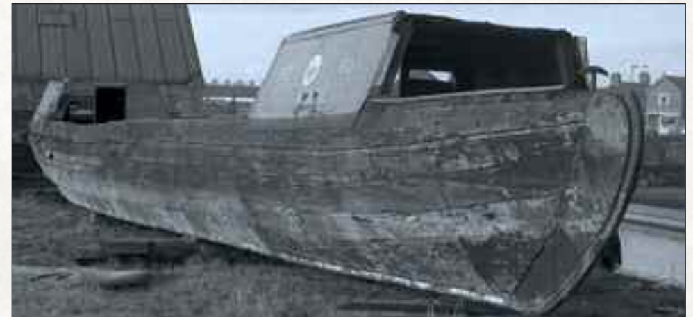
The fine lines of an ex. fly-boat subsequently used as a BW maintenance craft and named 'Etruria', photographed on 5 February 1967. It was one of the boats sunk by BW in the flash below Middlewich and subsequently raised by someone and put on the bank. According to records we have 'Etruria' was not its original SUC name. Unfortunately, I didn't get chance to measure it, but by its lines it could have been a Trench-fly. Any further information on the fate of this boat would be most welcome. Harry Arnold, Waterway Images Collection
