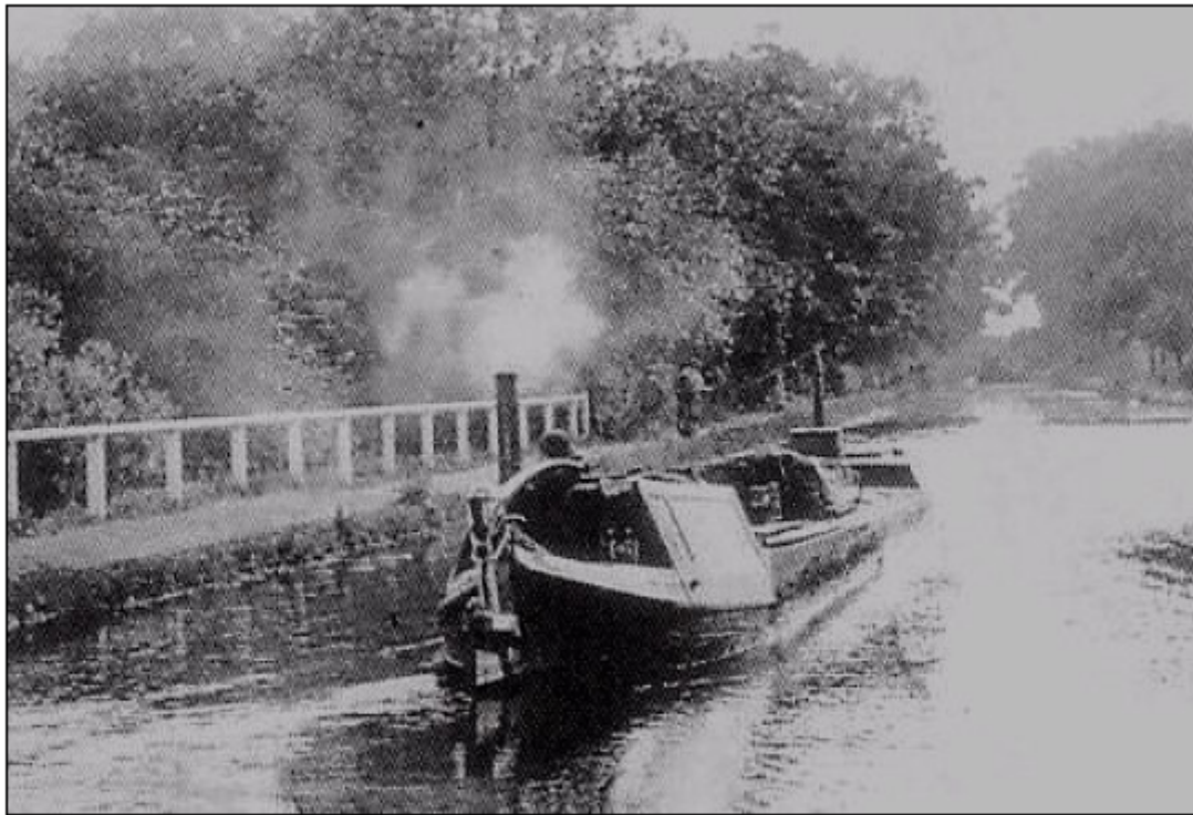
The horse drawn small tar boat 'Medina' at Newport. She was built narrow to go up Trench locks but mainly traded to Shrewsbury gasworks carrying waste acid to the Midlands.
